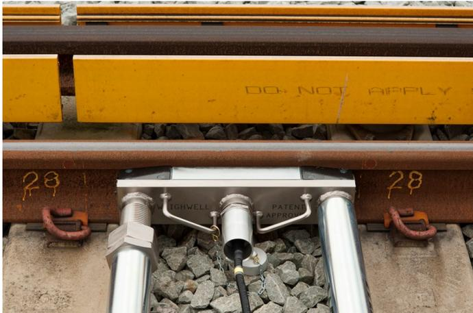
Our PTW allows for greater flexibility without the need to remove rail fastenings due to its length of only 500mm. This results in a more convenient installation and less 'flexing' of the system. The benefits of this are more accurate and reliable weighing results than your ordinary train weighing systems.
